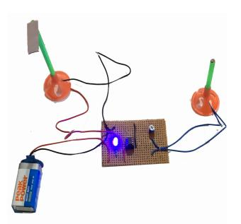
LDR Sensor Based Automatic Street Light Control Ready to Use Kit on Dotted/multipurpose PCB board
