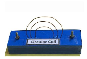
Magnetic field due to a current in a circular coil || Physics & Electromagnetism Experiment (Using Component Blocks)
