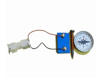
Electromagnet || Locate the Position of "Pole" of a Electromagnet || Physics & Electromagnetism Experiment (Using Component Blocks)
